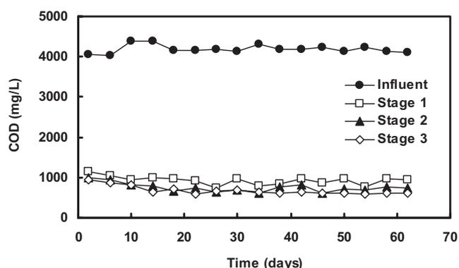
**Figure 2:** COD profiles of the three-stage biofilm reactor treating pyrethroid pesticide wastewater at a reactor HRT of 48 h.
