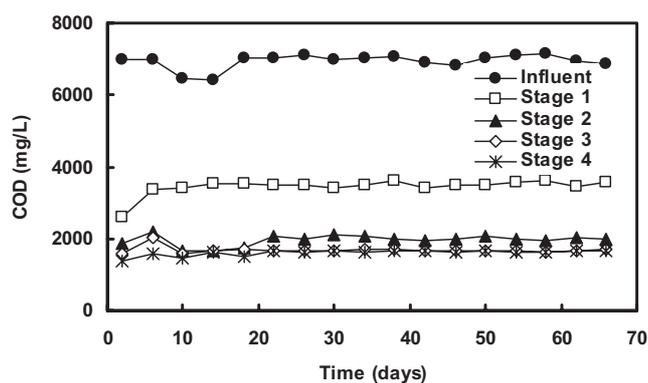
**Figure 4:** COD profiles of the four-stage biofilm reactor treating organophosphorus pesticide wastewater at a reactor HRT of 72 h.
