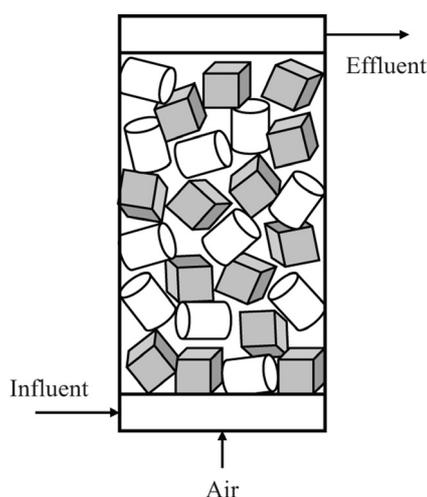
**Figure 1:** Dual media biofilm reactor packed with polyurethane foam blocks and cylindrical rigid spacers.
