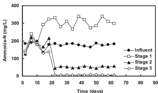
**Figure 3:** Ammonia profiles of the three-stage biofilm reactor treating pyrethroid pesticide wastewater at a reactor HRT of 48 h.
