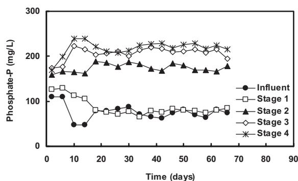
**Figure 6:** Phosphate profiles of the four-stage biofilm reactor treating organophosphorus pesticide wastewater at a reactor HRT of 72 h.
