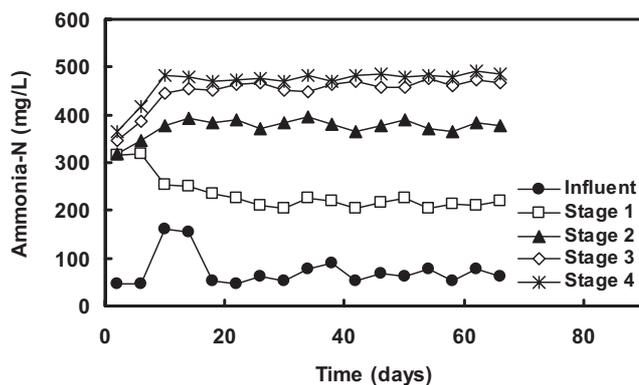
**Figure 5:** Ammonia profiles of the four-stage biofilm reactor treating organophosphorus pesticide wastewater at a reactor HRT of 72 h.
